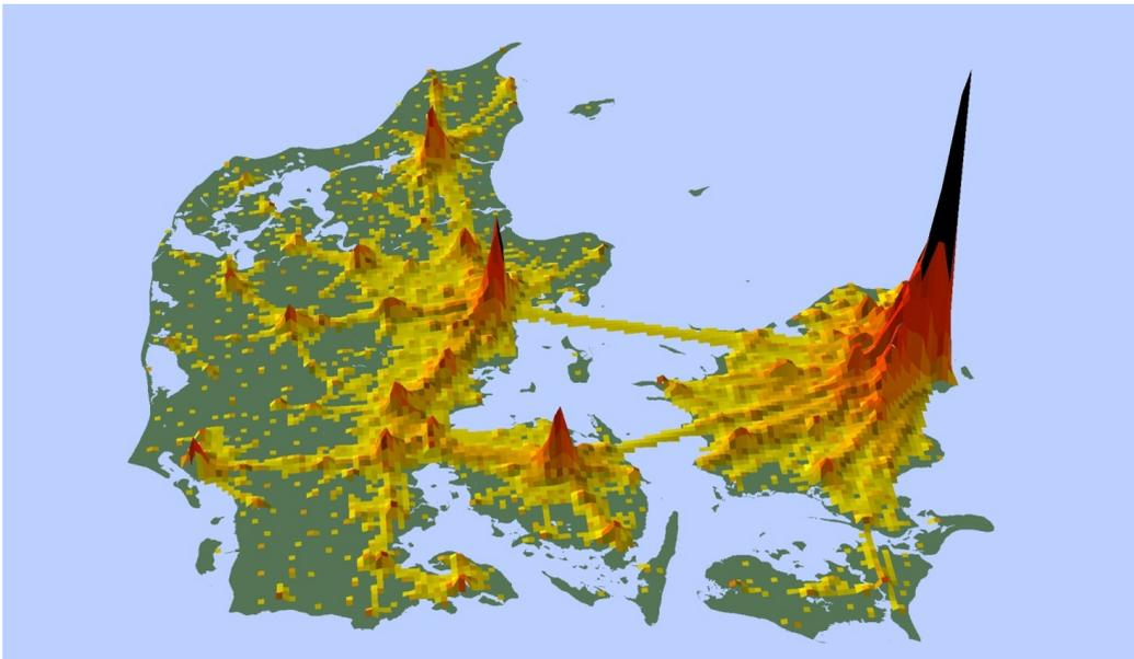
**Figure 1** Commuter flow or 'desireline traces' drawn from commuting in Denmark. The map is based on origin-destination data for commuting and summarizes the number of commutes passing through any given area.
